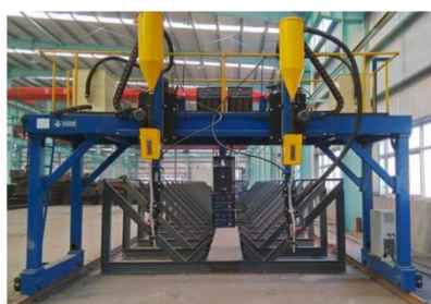
H-Beam Production Line
