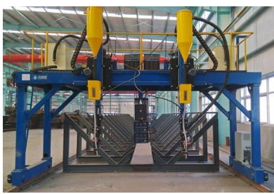
H-Beam Production Line
